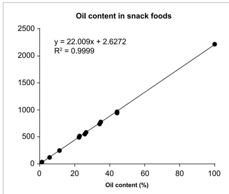
**Figure 1:** Correlation between NMR signal/mass and reference values
